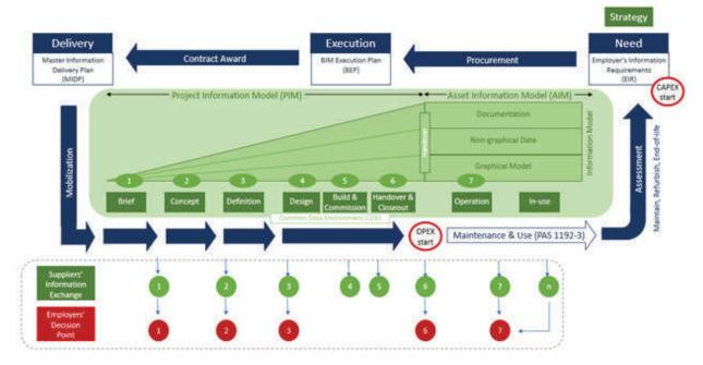
The above figure illustrates the project life cycle in a systematic way from brief to delivery the proper implementation of BIM. BIM can save the lead time and cost in terms of capital/operation expense optimally.
